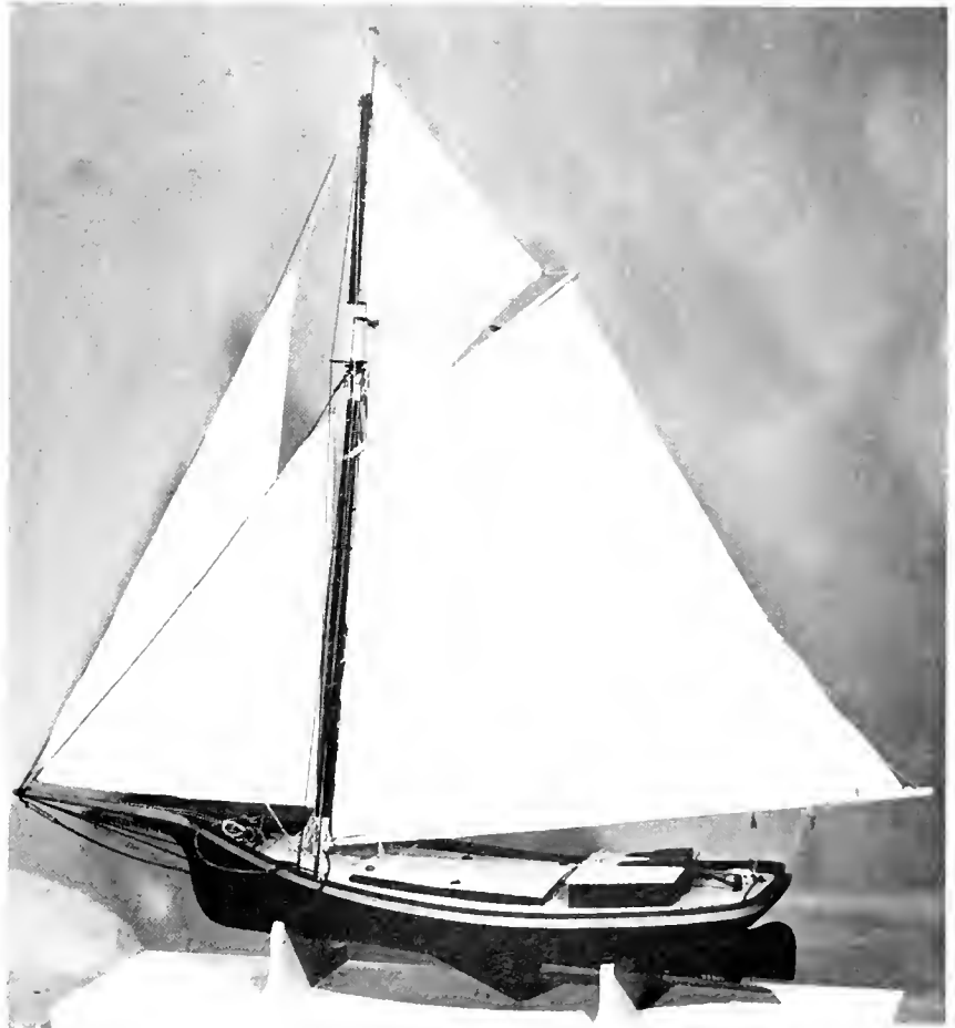
CENTERBOARD STEEPLE used as carry-away boat in the menhaden fishery on Long Island Sound in the 1870's. Rigged model USNM 57929. (Smithsonian photo 45607 c.)
